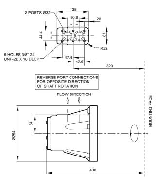
2 1/4" VALVE HOUSING WITH 1" SAE 4-BOLT FLANGES, F2'/FM2'
