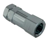
Standard unidirectional check valves, acting as a safety device into hydraulic systems. Standard versions contain a spring set to open the valve at 35 kPa; Normally available with inlet and outlet Female threads. Available sizes: 1/4", 3/8", 1/2", 3/4", 1", 1-1/4", 1-1/2", 2". Wide range of calibrations available, from 10 to 950 kPa.
