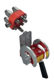
MultiFaster for High Pressure applications. 4 lines size o6. Working Pressure: 46 MPa. Flow rate @ 0.2 MPa: 35 l/min.
