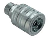
Female couplings designed for panel mounting installation and connection to flexible hoses. Wide range of threaded adapters available. Size 1/2". Interchangeable according to ISO 7241 Part A. Flow rate @ 0.2 MPa: 75 l/min.
