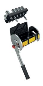
MultiFaster 10 lines, size 04. Working Pressure 25 MPa. Flow rate @ 0.2 MPa: 20 l/min.
