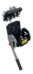
MultiFaster 12lines. 10 lines size 08, 2 lines size 04. Working Pressure 25 MPa. Flow rate @ 0.2 MPa: 10 lines 70 l/min, 2 lines 20 l/min.
