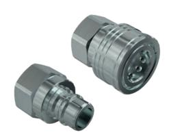
Male and Female couplings, suitable for Oil & Gas applications. Free Flow couplings. Designed to maximize flow, assembled without internal valves. Available sizes: 1/4", 1/2", 3/4". Interchangeable with Faster TNV couplings. Available also in brass (sizes 1", 1-1/2").
