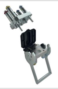
Multifaster 5 lines. 3 lines size o6, 2 lines size o9, 1 housing for electrical connector. Working pressure 22 MPa. Flow rate @ o.2 MPa: 3 lines 20 l/min, 2 lines 35 l/min.
