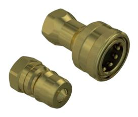
Male and Female couplings for industrial applications with poppet valve shut-off system. Brass version available with NBR or Viton seals. Available sizes: 1/8", 1/4", 3/8", 1/2", 3/4", 1", 1-1/2". Interchangeable according to ISO 7241 Part B.
