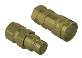
Flat Face Male and Female couplings for industrial applications. Brass version with seals in Viton. Available in size 1/2". Interchangeable according to ISO 16028.
