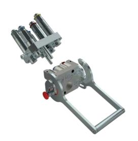
Multifaster 5 lines. 2 lines size o6, 3 lines size o9, 1 housing for electrical connector. Working pressure 25 MPa. Flow rate @ o.2 MPa: 2 lines 20 l/min, 3 lines 35 l/min.
