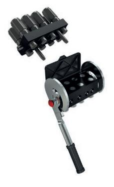
MultiFaster 8 lines, size o8, "G" type, with greaser and Zinc-Nickel plating. Working pressure: 25 MPa. Flow rate @ 0.2 MPa: 70 l/min.
