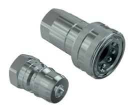
Male and Female couplings for industrial applications with poppet valve shut-off system. Available sizes: 1/8", 1/4", 3/8", 1/2", 3/4", 1", 1-1/2", 2". Complete range of sizes available with BSP, NPT and SAE Female threads. Interchangeable according to ISO 7241 Part B.
