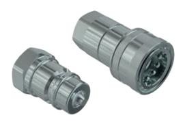
Male and Female couplings with poppet valve shut-off system. Size 1/2" interchangeable according to ISO 7241 Part A. Flow rate @ 0.2 MPa: 75 l/min.
