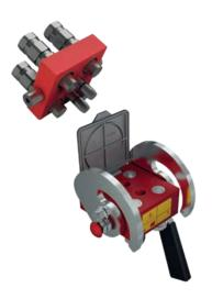
MultiFaster for High Pressure applications. 4 lines size o8. Working Pressure: 46 MPa. Flow rate @ 0.2 MPa: 60 l/min.
