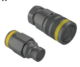
Flat Face Male and Female couplings, suitable for High Pressure applications. Flat valve shutoff system prevents contamination and spillage. Zinc-Nickel plating ensures good resistance to wear and corrosion. Maximum Working Pressure: 72 MPa. Available sizes: 1/4", 3/8".
