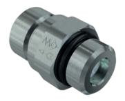
Compact check valves, acting as a safety device into hydraulic systems. Very compact design, assembled with only one piece body. Standard cracking pressure 35 kPa. Available sizes: 1/4", 3/8", 1/2", 3/4", 1".
