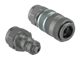
Male and Female couplings for Ultra High Pressure applications. Working pressures of 100 MPa. Very robust and reliable, equipped with safety sleeve. Characterized by redundant visual and mechanical safety systems. Available in size 1/4". Red caps provided as standard with the couplings.
