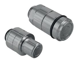
Flat Face Male and Female cartridge couplings in Stainless Steel (AISI 316) with Viton seals. Self-aligning couplings for MultiFaster. Misalignments up to  $\pm$  0.5 mm and  $\pm$  1° (angular) are automatically compensated during the connection. Available sizes: 1/4", 3/8", 1/2". Faster proprietary profile.
