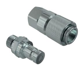
Diagnostic Flat Face Male and Female couplings, specifically designed to measure the internal pressure of hydraulic circuits. Male part to be mounted on the hydraulic line, Female part to be connected to gauge instruments. Available in size 1/4". Interchangeable according to ISO 15171-1.
