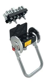
MultiFaster 10 lines. 5 lines size 08, 5 lines size 04. Working Pressure 25 MPa. Flow rate @ 0.2 MPa: 5 lines 70 l/min, 5 lines 20 l/min.
