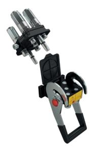
Multifaster 5 lines. 3 lines 04, 2 lines 06. Working pressure 25 MPa. Flow rate @ 0.2 MPa: 3 lines 20 l/min, 2 lines 40 l/min.
