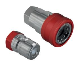
Male and Female couplings with poppet valve shut-off system, Lloyd's certified, suitable for Oil & Gas applications. Thanks to special components and seals, HNVFR couplings are API 16 D certified and suitable for BOP application. Available sizes: 1/2", 3/4", 1". Interchangeable according to ISO 7241 Part B.
