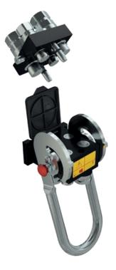
MultiFaster 4 lines. 2 lines size 08, 2 lines size 12. Working pressure: 25 MPa. Flow rate @ 0.2 MPa: 2 lines 70 l/min, 2 lines 105 l/min.
