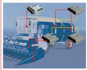
Fig. 17: Decentralized control architecture using the example of a combine harvester
