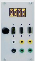
The data interfaces of the connected controller can be tested using the communications module. Specifically using the CAN interface, it is possible to enable termination resistors and to switch short circuits to other states.
