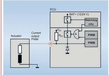
One problem when operating proportional valves with solenoid coils is that the solenoid coil increases its resistance as it heats up. This increase in internal resistance has the effect of reducing the coil current for the same supply voltage. Since the coil current is in turn proportional to the positioning force of the solenoid, the spool position of the valve also changes. To counteract this shift in the hydraulic operating point, the coil current can be measured and thereby also controlled.
