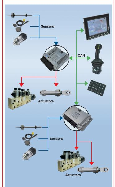
Fig. 20: Centralized structure using a controller and an I/O expansion module
