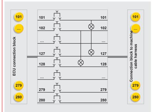
Using the 2 mm bridging connector with test points, the actual signal levels for each pin on the controller can be accessed. Additionally, by removing the bridging connector, external signals can be connected to the wiring harness.
