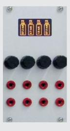
The sensor supply simulation module allows the sensor power supply supplied by the ECU to be tested. It is thus possible to measure the real-time voltage as well as the current. In addition different error signals can be switched.
