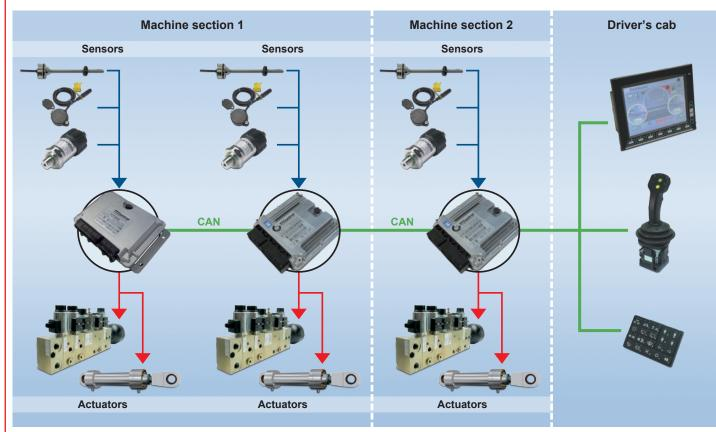
Fig. 21: Decentralized structure with two controllers and an I/O expansion module
