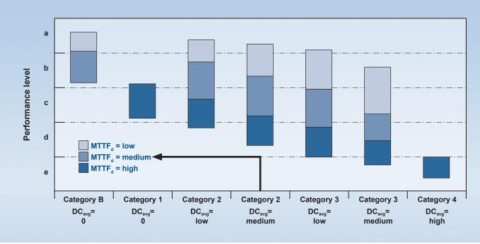
Fig. 30: Determining the PL using the bar chart
