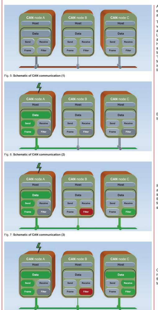
Fig. 8: Schematic of CAN communication (4)
