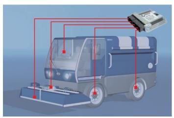
Fig. 16: Centralized control structure using the example of a municipal vehicle
