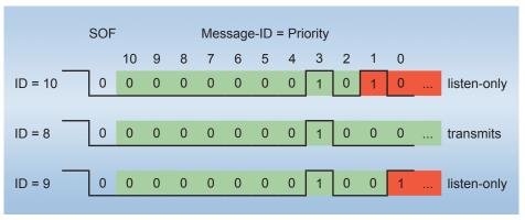
Fig. 13: Arbitration of transmission rights
