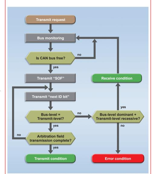
Fig. 14: Bus access using CSMA/CA
