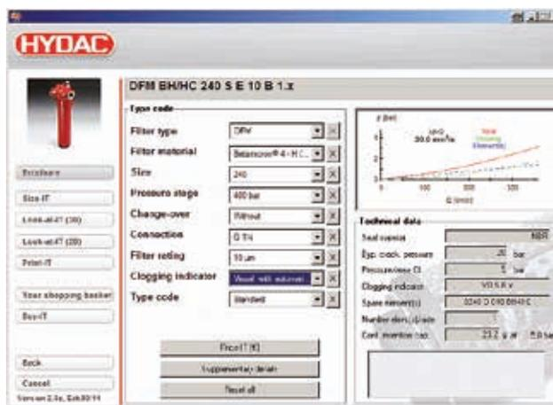
**Filter calculation according to the expected contamination rate using the concept creation tool "Optimize-IT"**
