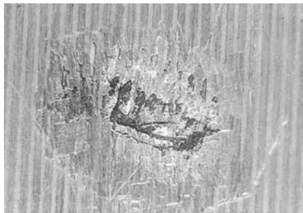
Surface fatigue on ball bearing
