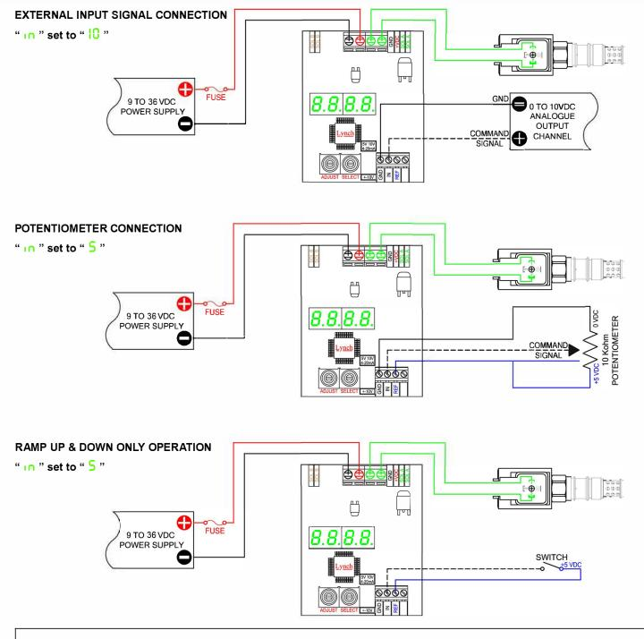
**PLEASE NOTE:** For "0 to 5 VDC" & "0 to 10 VDC" command input drivers, it is recommended to use independent negative conductors for power supply and analogue output channel (PLC/PC) to maintain command signal accuracy due to voltage drop on long cable runs.
