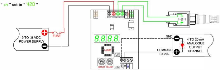
TWO WIRE TRANSMITTER INPUT CONNECTION
